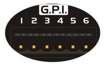
The connections on this port also include a 3V3 output for use with all logic or analogue level inputs. For ground (0V) connections, this must be derived from the RS485 "Phoenix" connector.
