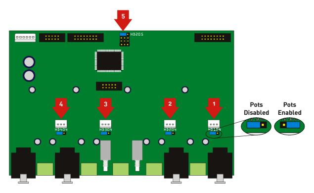
HD104 disables the pot for channel A, HD204 disables the pot for channel B, and so on, with HD205 setting the pot enabled/disabled flag, the state of which can be monitored remotely though iCore.
