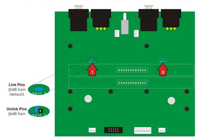
When selecting the 36dB gain position, we recommend fitting the jumper link back onto one of the individual pins for storage, in case the gain has to be changed back at any stage.
