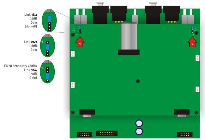
\*Equivalent gain for the fixed sensitiviy setting is 39dB.
