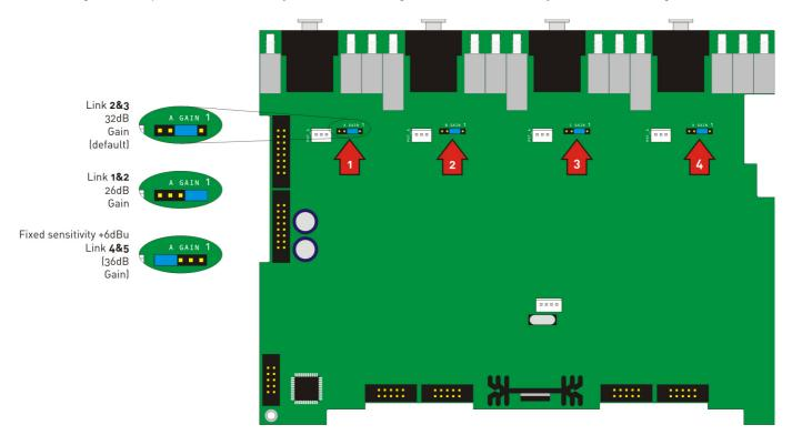
\*Equivalent gain for the fixed sensitiviy setting is 36dB.
