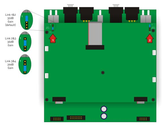
Remember, setting higher gain does not change the maximum available power but changes the level of signal input to achieve maximum power. In any case, provided that the input signal is less than 20dBu/7.7V, the built-in limiter circuit will prevent distortion within the amplifier.
