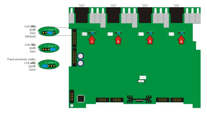
Remember, setting higher gain does not change the maximum available power but changes the level of signal input to achieve maximum power. In any case, provided that the input signal is less than 20dBu/7.7V, the built in limiter circuit will prevent distortion within the amplifier.
