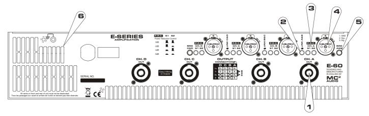
1: Channel A output Speakon socket: Normal output is on pins 1+ hot, 1- cold. Channel B's output is also wired to this socket to enable a single NL4 to provide both channels and to facilitate easier wiring in bridged mode. Channel B is wired pins 2+ hot, 2- cold.
