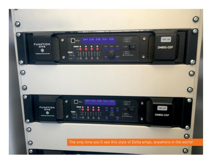
And a lot of them. Over 200 channels worth (over 50 amplifiers) totalling close to half a megawatt of power. As all but one of the amplifiers (?!) needed to have processing, the amps were a mix of Delta 80 and Delta 100 DSP models. There was also a mysterious single non-DSP Delta Series amp – fitted with Dante but not required to have remote control...more on that later!
