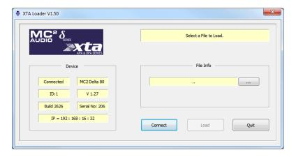
Click the "Connect" button, the software will scan all available connections and search for connected amplifiers.
