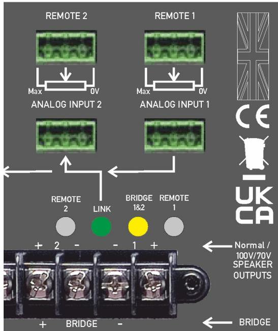
Your amplifier can source audio from analogue or network locations (if a network card is fitted).
