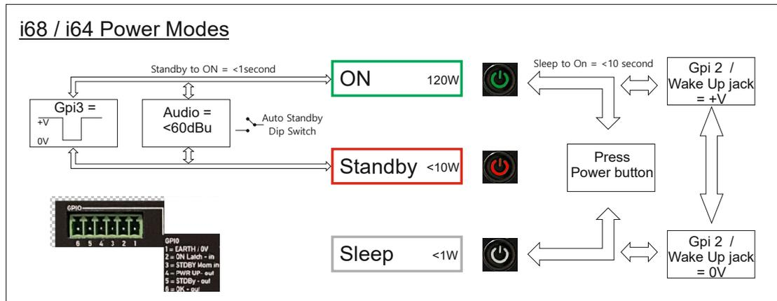
Your amplifier has 3 power modes On, standby and sleep. There are various method to move between these modes – these methods are displayed in the above diagram.
