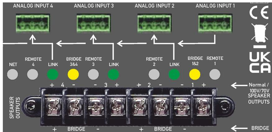
Your I series amplifier allow easier connection of hi z and lo z speaker via the rear barrier strips. **The DIP switches which change Lo Z and Hi modes should only be operated when the amplifiers is OFF/ SLEEP.**
