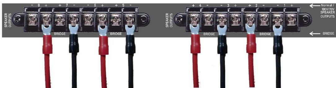
When operating in bridged mode, the minimum impedances are doubled.
