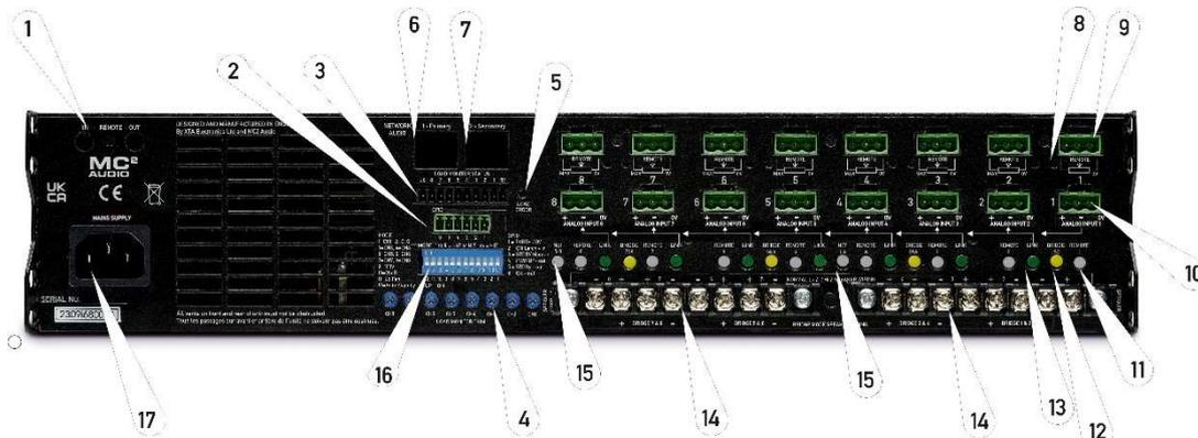
**1: Remote: 3.5mm stereo jack** input and output for remote enabling power on / sleep. This is normally high, Pull low to switch OFF/SLEEP. For example connecting the tip / ring of the 3.5mm jack to each other will enable sleep.
