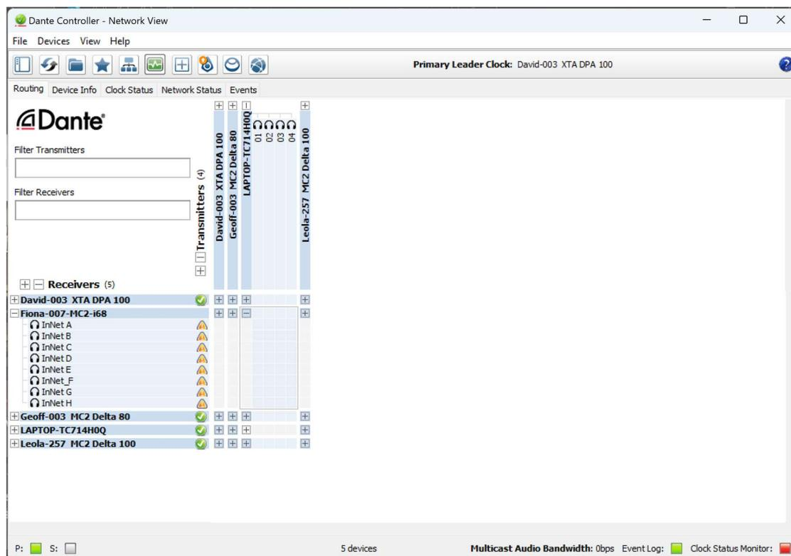
Note that the rear panel “Link” switches do not function on the Network Audio inputs. If linking is required this can be set up as part of the source selection within Dante Controller.
