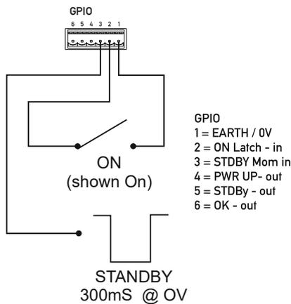
Last takes precedence rules apply to Power button, Wake up Jack, GPi 2 and GPi 3 logic.
