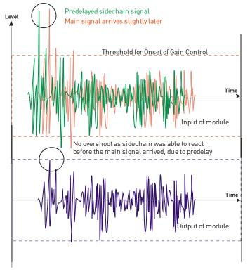
The pre-delayed sidechain is shown in green, with the main signal in red. As the main signal arrives slightly after the sidechain, the output from the unit does not suffer from the overshoot problem.
