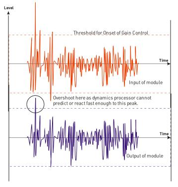
For an analogue dynamics processor, the situation is much better. Controlling the gain electronically, and not relying on a human sidechain feedback mechanism, it can react much more quickly.
