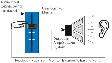
Feedback Path from Monitor Engineer's Ears to Hand forming Sidechain Control Signal
