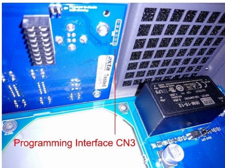
The lowest hole (one nearest the bottom, by the tested sticker) is marked with a dot – this is pin 1.
