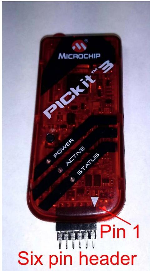
If not already inserted, plug in the 6 pin header as shown here. Also, note the marker to show pin 1 of the interface – this is required to align with the correct polarity of the programming interface on the front panel circuit board.
