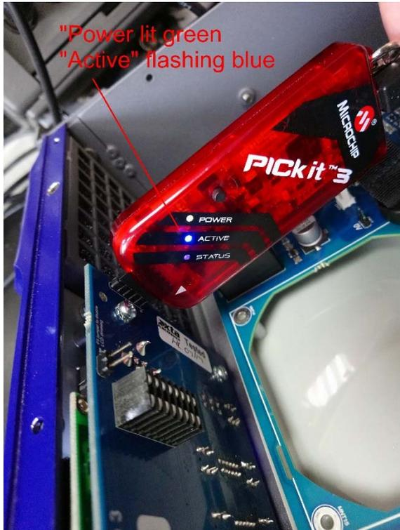
Insert the programmer into the header as shown, so that pin 1 on the programmer is connected to the lowest hole. **It is NOT necessary to remove the fan as in the photographs – this has been removed for clarity.**
