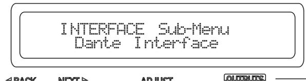
Use the encoder or BACK and NEXT keys to find the Dante Interface option and press ENTER. If the screen shows a message...
