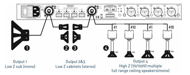
Remember that the Delta 20 and DNA20 is a quad channel amplifier and so there's no reason why the audio for the ceiling speakers in the restaurant has to be the same as that for the bar.
