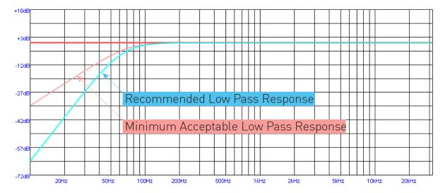
The DNA20 and Delta20 have this HPF built-in, and this is activated (on an individual channel basis) on channels with transformers fitted.
