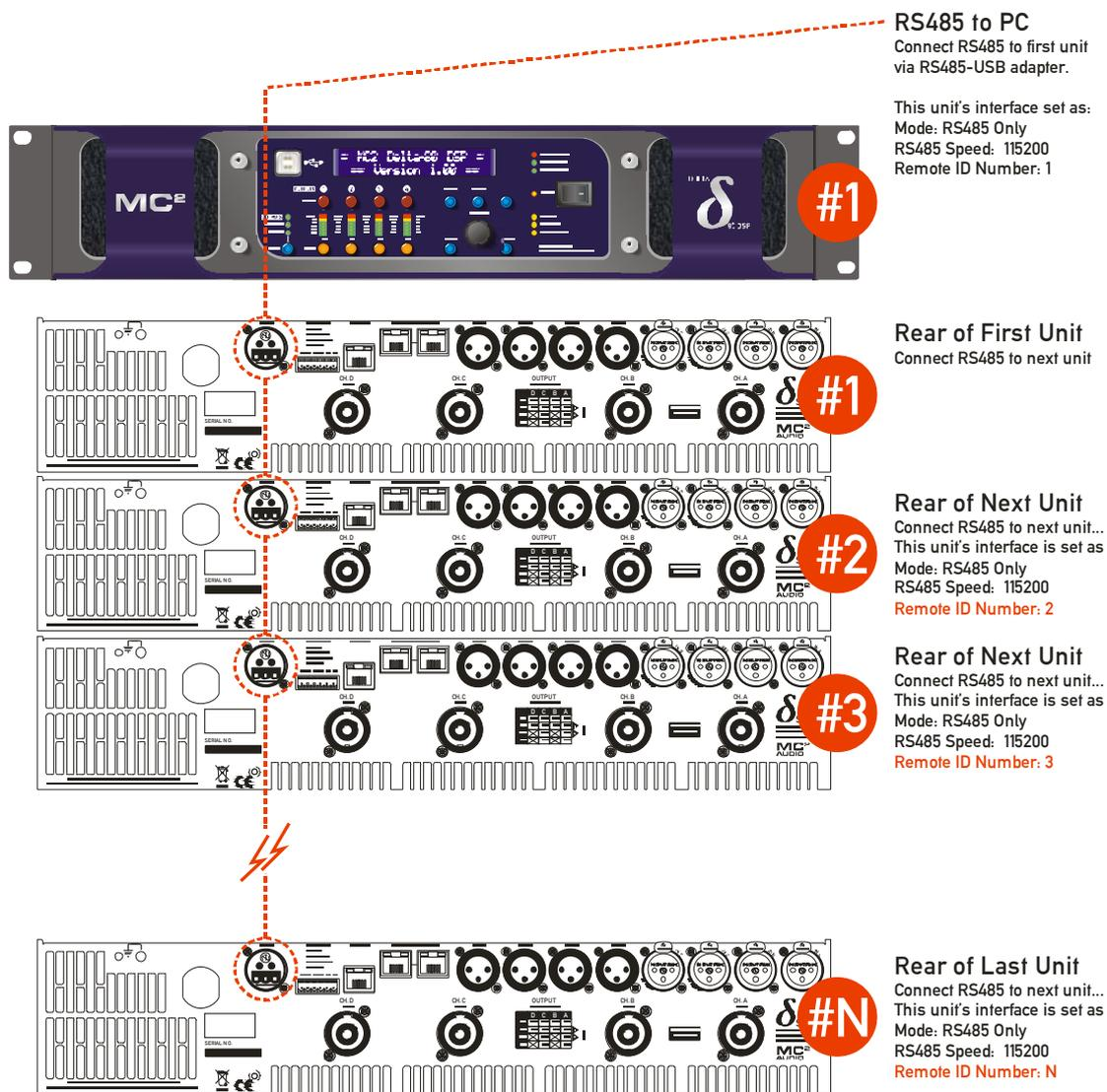
Remember that APA amplifiers cannot connect via RS485 (despite having the RS485 socket on the rear panel – this is for test diagnostic purposes only)
