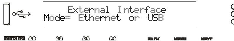
Use the encoder or BACK and NEXT keys to choose the required interface and press ENTER. This will invoke a series of further options depending on the interface chosen – these are explained below:
