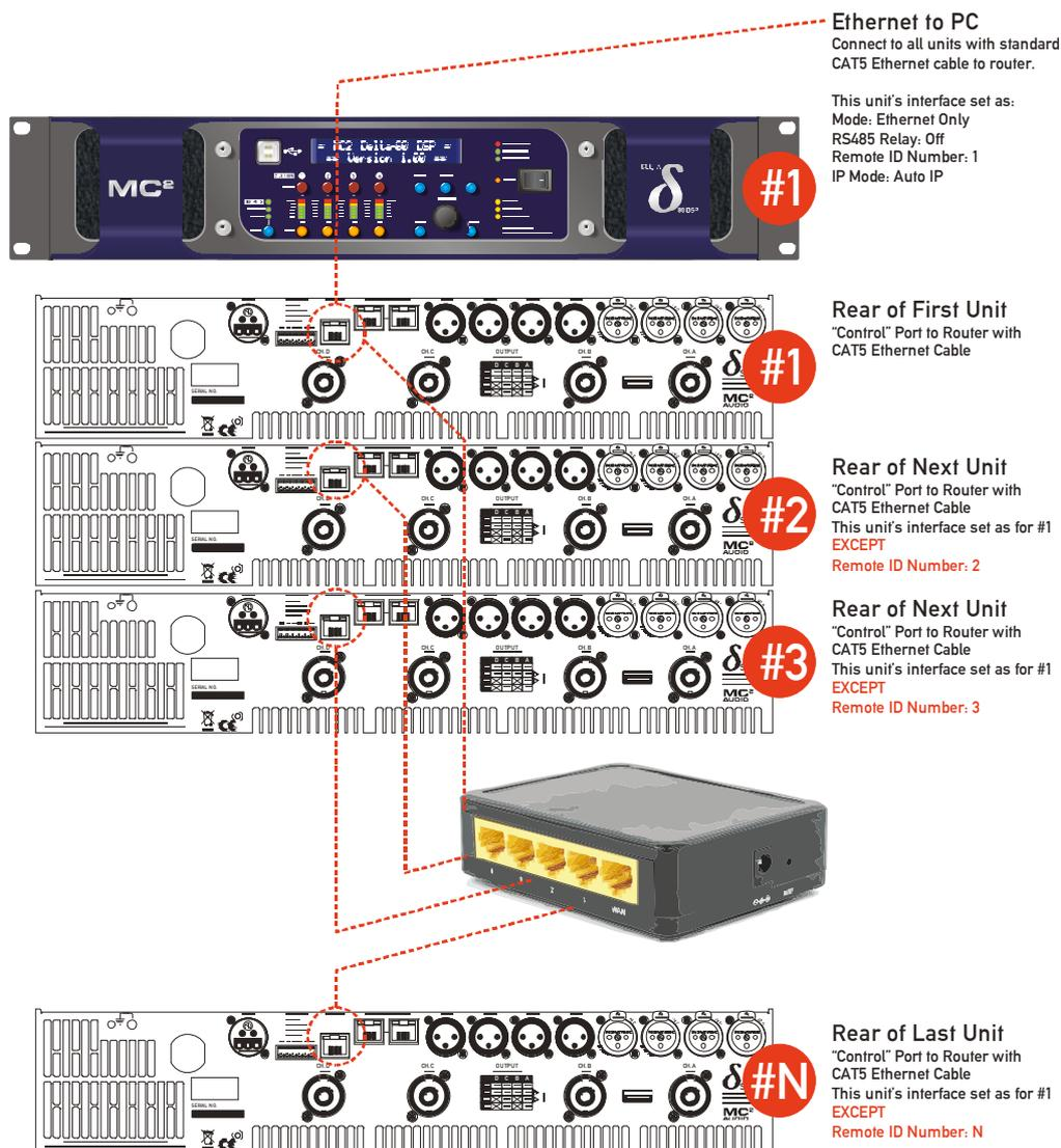
Remember that the recommended max distance for a point to point Ethernet connection is 100m – beyond this a switch must be used to extend the distance. Make sure that there is only one DHCP server on a network if multiple switches or routers are being used (especially if a Wifi router is connected as well).
