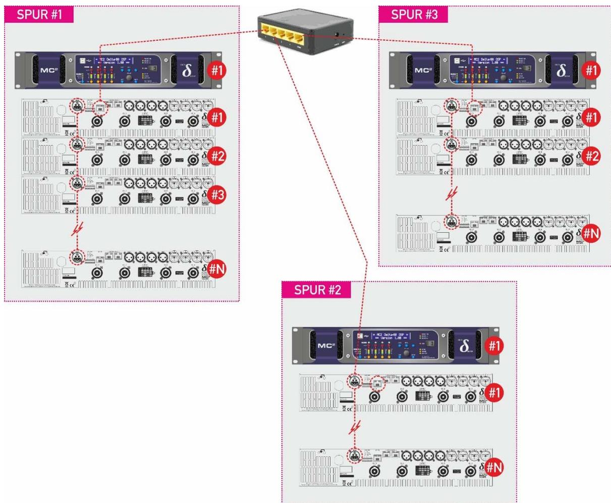
Note that the total number of IDs on the system must not exceed 32 amplifiers, and that ID numbers cannot be repeated, even on the individual spurs as in the example system above.
