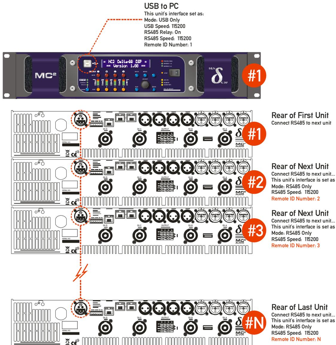
The only disadvantage is that this connection method cannot work with DeltaDirect – our iPad app, as there is no way to establish a wireless control connection. Remember that the total length of an RS485 bus is 1000m from the first device to the last – not 1000m per interconnect!
