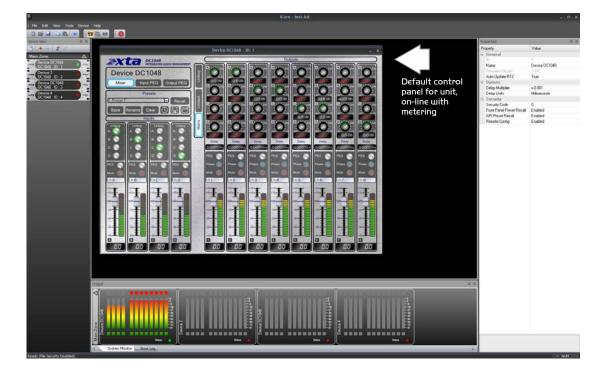
In the example on the previous page, all devices apart from the first one are offline, as shown by the red indicator on each unit in the Device View and the System Monitor view. When connected and on-line, the indicators will be green. A yellow flashing indicator means there is a problem – hover over the device in question to see a tool tip explaining what is wrong.
