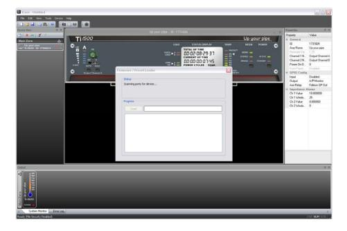
The loader will start scanning for all connected devices to determine what unit it has to update. After a few seconds the device will be found and identified (its Power LED will begin to flash). Check the model number, which will be shown in the status pane and if OK, press the "Load" button.
