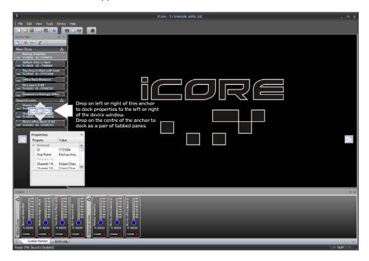
To separate out the windows again, just click on the tab of the window and drag and drop it as required to select a new position.
