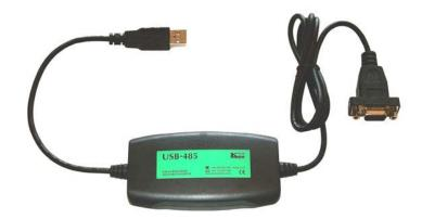
This device is powered via the USB connection and so has the ability to drive long cable runs reliably. This device is available from us, or directly from KK Systems at <a href="https://www.kk-systems.com">www.kk-systems.com</a>. The converter comes with a 9-pin D-type fitted as standard – this has to be adapted to an XLR connection.
