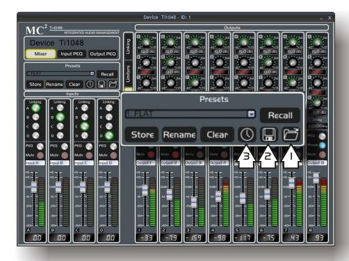
Storage of presets within the unit is accomplished by selecting the required location from the drop-down list and then choosing Store. Recall is instantaneous with all settings changing on the unit and updating on the software control panels. Storing settings will pop up a window allowing the name to be changed before storing, and renaming allows just the name of a preset to be changed without saving new settings.
