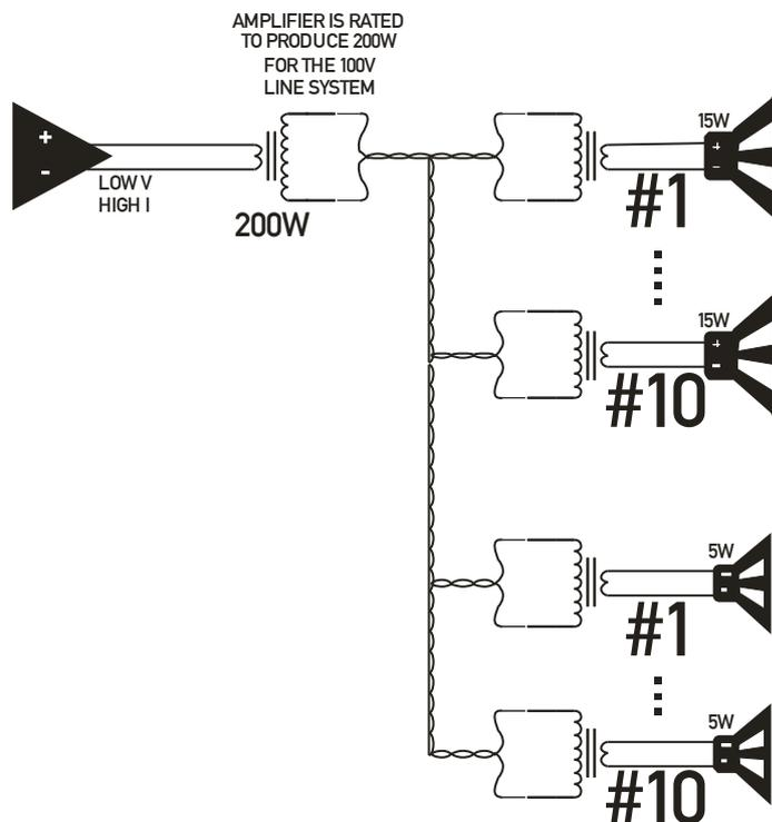
Let's say we have worked out that we need 10 of the 15W speakers, for starters – that comes to  $10 \times 15W = 150W$ , leaving us with 50W "spare", which means we could connect another 10 of the 5W speakers. That's 20 areas in total – not bad for just 200W!
