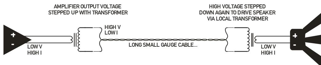
Once the voltage has been “stepped up” to the higher level for long distance transmission, when it reaches the speaker, in common with mains power reaching its destination, there must be some form of “stepping down” again to restore it to a voltage/current suitable for driving the speaker. This is achieved by using a localised “step-down” transformer, normally attached directly to the speaker chassis itself, or in the enclosure with the driver.
